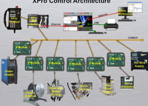
The XPro utilizes multiple processors that are dedicated to each welding function and networked together to share all process information. This architecture allows the ability to provide tightly integrated systems in which all motion, power supply, and sensor functions are programmed and controlled from a single controller.
