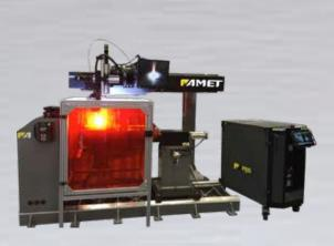
AMET Circumferential Welding System with XPro-Mobile weld controller
