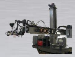
Tandem wire SAW and single wire GMAW system with motorized travel cart, laser seam tracking, flux delivery and recovery, and camera package for general manufacturing.
