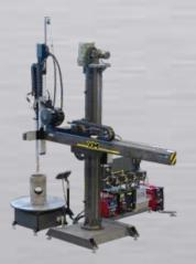
GTAW and GMAW manipulator with separate wire feeders for hotwire GTAW and cold wire GMAW, AVC on both Z and X axes. Includes intersecting bore cladding capability for manufacturing oil and gas industry components.
