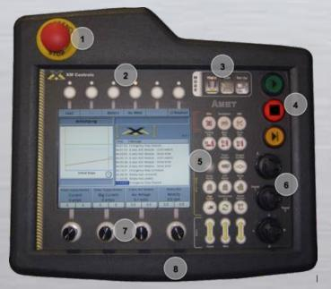
1. The Emergency Stop (E-Stop) button immediately terminates the weld program, stops weld current output from the power supply, and ceases all servo-controlled motion.
