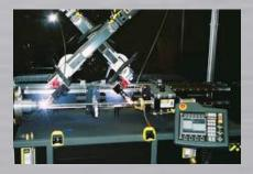
GTAW lathe with dual torch weld heads capable of performing welds at the headstock and tailstock simultaneously. Each weld head has touch retract and AVC capability.
