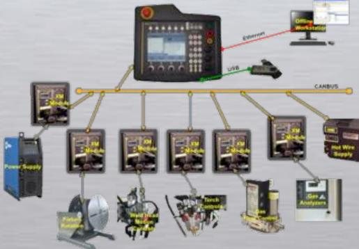
**Controller Configuration:** The XM Controller is networked with a group of control modules for complete welding system integration. Each XM control module has its own DSP (Digital Signal Processor) and communicates with the XM Controller through the CAN Bus network. The use of DSPs allows for real-time feedback and monitoring of the welding processes and motion control.
