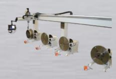
Sidebeam GTAW system with four precision positioners, laser seam tracking, AVC, wire feed, and 330 inches (8382 mm) of carriage travel.
