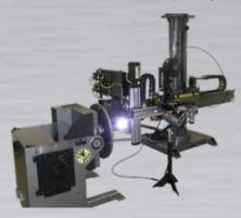
Precision GTAW manipulator system for repairing and manufacturing power generation industry valves.
