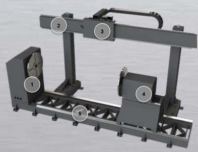
1. The headstock assembly provides programmable rotation for circumferential welding. The assembly is fixed into position at one end of the lathe base. A faceplate with four (4) tooling slots and a thru hole is included for adding specialized tooling or backing / purge gas capabilities.
